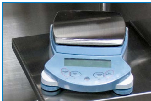
LW419 - ELECTRONIC SCALE - PLATFORM 6.6 in. x 6 in. Platform, 2100g. Compact, lightweight, portable and perfectly suited for laboratory and educational purposes. 2200 x .1 gm.
