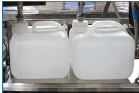
OA-201 - FORMALIN DISPENSING AND COLLECTION 2.5 gal. container and receptacle hold reserve formalin and collects waste. Foot controlled motor dispenses formalin at a steady flow.
