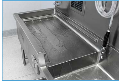
OA-116 - END RINSE ASSEMBLY Provides a constant flow of water beneath the dissecting area grid plates to wash debris toward sink and drain. Includes cold water control valve and back flow protection.
