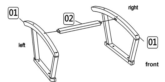
Ensure the longer side of Part02 is facing front and there is no gap between Part01 and 02.
