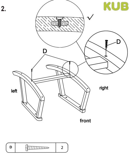
Ensure the screws are tightened and sit bellow the top surface of the countersunk holes.
