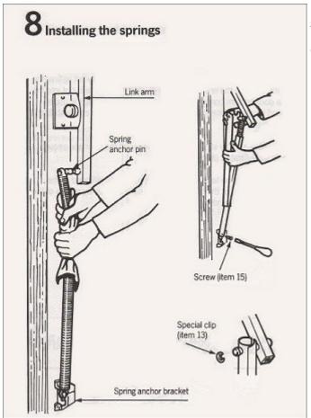
Finally, repeat the procedure for any additional springs, and ensure the door is operating correctly.
