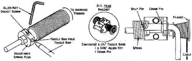
To reapply spring tension (if all or most tension has been lost).
