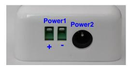
Using the screw plugs and DC on the input interface of the bridge. **DC Output:**
