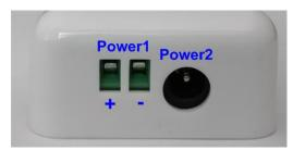
With screw plugs and DC on the input interface of the bridge
