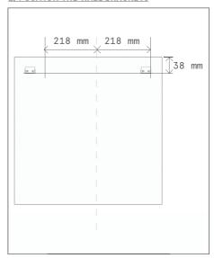
Measure out where to place the wall brackets from where the center and top should be.
