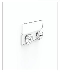
Attach the brackets to the wall with screws, but don't tighten the screws.
