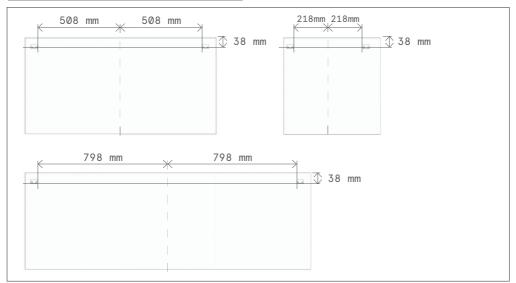
Depending on the size and orientation of each Basic Wall element, there are three alternative positions for the wall brackets. They are placed as described above.
