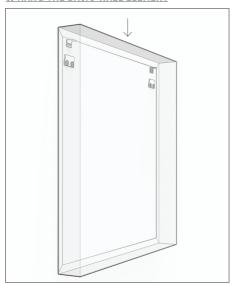
Place the BasicWall element a bit above the wall brackets, and slide it down into place.
