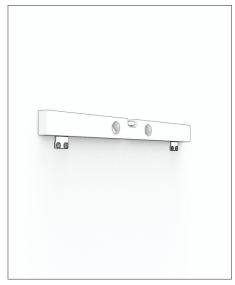
Use a leveler to straighten out and aline both wall brackets. Then tighten the screws.
