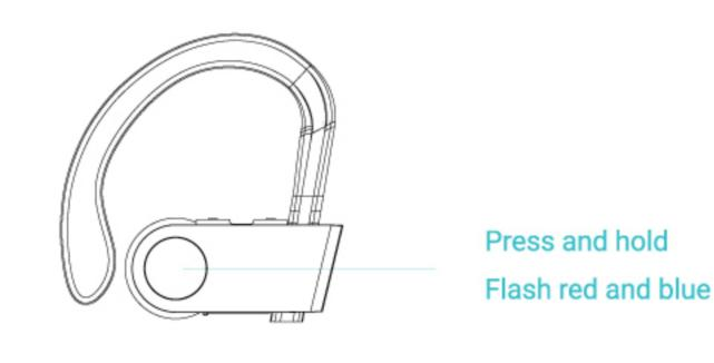
During charging, press and hold MFB until the indicator flashes red and blue alternately.
