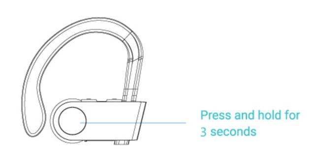
To enter pairing mode, press and hold MFB until the indicator flashes red and blue alternately. (The headset will directly enter pairing mode the first time you turn it on. To enter pairing mode for the next time, you need to follow the above mentioned steps.)
