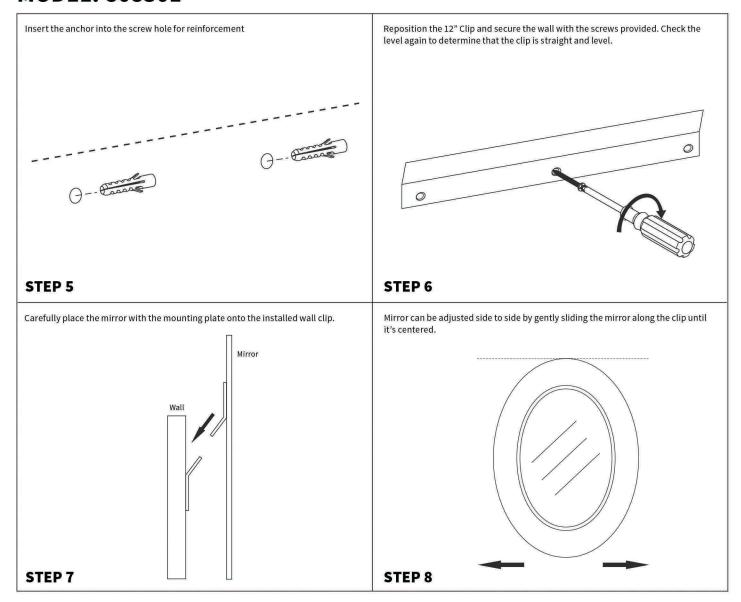
Licensed professional installation is recommended. These instruction are for mounting into studs or other in-wall reinforcement, drywall alone is not sufficient to support wall-hung vanities. Other installation techniques may require a licensed professional.
