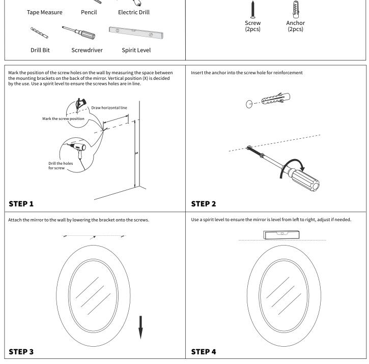
Licensed professional installation is recommended. These instruction are for mounting into studs or other in-wall reinforcement, drywall alone is not sufficient to support wall-hung vanities. Other installation techniques may require a licensed professional.
