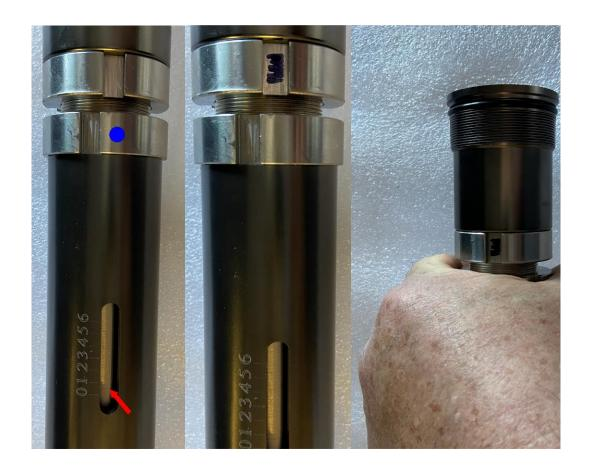
Turn until the adjustment mark (red arrow) lines up with the desired preload value.
