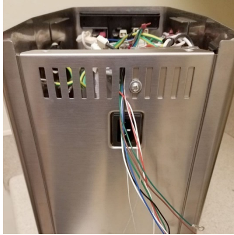
Figure 29. Feed all wires through the slot next to the SSR.
