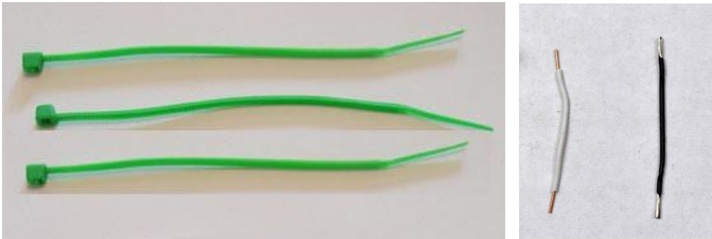
Figure 7. Cable ties (left) and the jumper wires (right). The white jumper wire is for the RTD sensor, and the black jumper wire is for the water-pump control.
