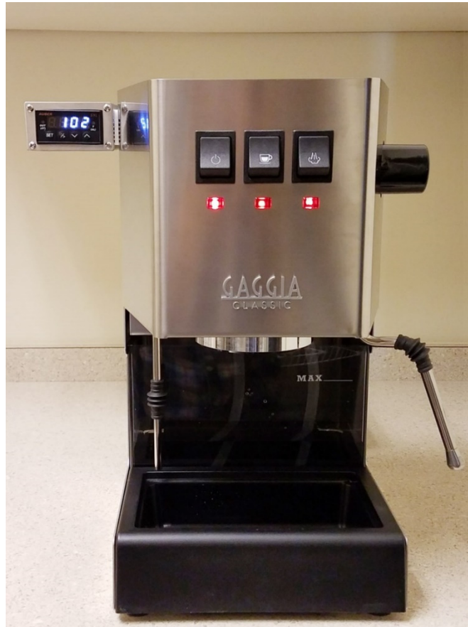
Figure 37. Gaggia Classic Pro (European model) with KIT-GGP (white LED display) installed.
