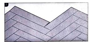
The boards need to be locked into one another, using the click lock system. To connect a new board you have to use a rubber hammer.
