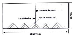
Lay out the triangles with their long side towards the starting wall. Align the center triangle top with the installation line.
