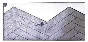
Use a rubber hammer and slightly knock at the click lock system to connect the short side. Start in the corner and work towards the end of the board.
