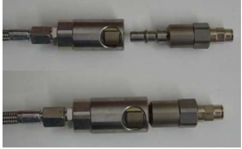
Top is QD (quick disconnect) apart/disconnected. Bottom is together/connected Because of the pressure it will take some effort to push them together to connect. So keep that in mind when deciding where to place it and or line length. When reconnecting you will get a small amount of leakage.
