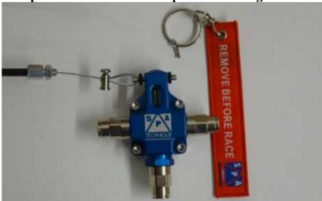
Note, Bracket will need to be made to hold pull cable housing (outer sheath). Also far enough away to allow the cable pull the pin out. Also as straight/in line with the pin as possible Otherwise the pull cable will not work. Also it could be done like in the previous configuration or for a second pull cable.
