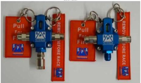
Optional compression fitting (left) for steel tubing from bottle/cylinder to block Optional -6 fitting (right) for steel braided line
