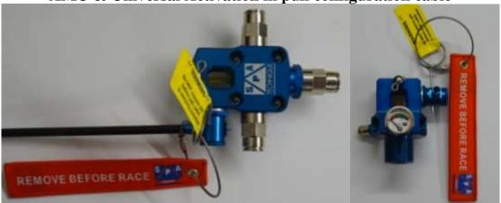
Note, mechanical activation piece can be threaded into either side of the activation head and/or a second mechanical, or another activation type, can be utilized, as well. Also do not remove safety pin until pull cable is in place as shown on the left/AMU block. In the left picture you can see the cable needs to just come out. If you need to cut the cable down you will need to silver solder it or zap the end with a tig welder to keep it from fraying.
