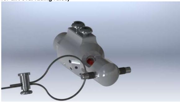
Bracket will need to be made to hold pull cable housing (outer sheath). Otherwise the pull cable will not work. Pull as straight as possible/in line with the pin. Or cable can be looped around just the thermal bulb. Make sure there is enough room between cable loop to cable housing to pull pin out or break bulb when pulled.
