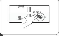
Carefully pour in the rinse-aid into its dispenser, whilst avoiding it to overflow.
