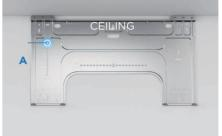
STEP 1: Mark the SPOT A according to the intruction of scale-on-plate
