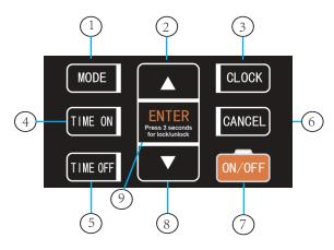
Only in unlocked state, pressing the button is functional.
