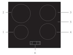
1. Max. 1300/1500W zone 2. Max. 2300/2600W zone 3. Max. 1800/2000W zone 4. Max. 1800/2000W zone 5. Glass plate 6. Control panel
