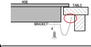
Under any circumstances, the brackets cannot touch with the inner surfaces of the worktop after installation (see picture).
