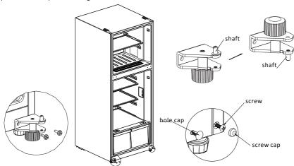
5)Dismantle the stoppers, sleeve pipes of both refrigerator door and freezer door, install them on the other side of both doors; exchange the installation position of sleeve pipe and hole cap on upper end cap of refrigerator door; remove the left decorative cover of freezer door, and move the sleeve pipe
