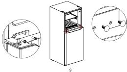
7) Take out the left upper hinge, left upper hinge cover, and right decorative cover from the accessory bag, install the freezer door on the middle hinge, and install the left upper hinge, left hinge cover and hole cap. Finally, install the right decorative cover on right side of end cap of freezer door..
