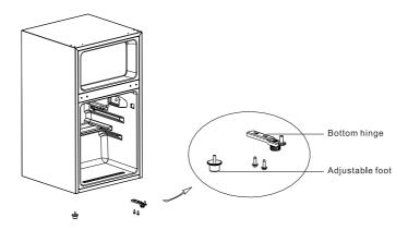
5) Exchange the installation position of bottom hinge and adjustable foot, then fix them respectively. Remove the hinge sleeve pipe of the refrigerating chamber door, and install it on the other side. Remove the hinge sleeve pipe of the freezing chamber door and install it on the other side.
