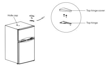
3)Remove freezer chamber door as well as middle hinge and hole cap of the other side.
