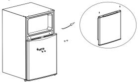
7) Place freezer chamber door on middle hinge ,then fix the top hinge,top hinge cover on left side and insert hole caps on right side.
