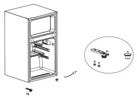
6)Place refrigerating chamber door on bottom hinge, then fix the middle hinge on left side and insert the hole caps on right side.
