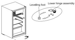
4)Install the door on the lower hinge assembly, and then install the upper hinge, hinge cover, shaft sleave , pins and hole cap in sequence.
