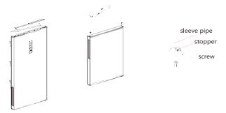
6.Put the freezer door on bottom hinge, install the middle hinge, the screws and the screw hole caps.
