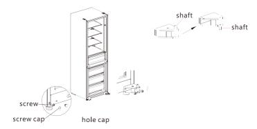
5. Dismantle the screws, sleeve pipe and stopper on the lower end cover of the two door bodies, and install them successively on the other side of the door bodies (the stopper needs to be replaced from the additional bag). Then remove the upper end cover of the cooler door and switch the wire harness with a sleeve pipe to the other side of the door body. Finally install the sleeve pipe of the upper hinge on the cooler door in the hole on the other side of upper end cover of the cooler door.
