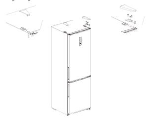
3. Dismantle the middle hinge, the screws ,the screws hole caps and remove the freezer door.
