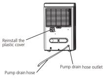
• Press the pump pad of the unit to activated the pump operation. When the bucket is full the pump starts to work.
