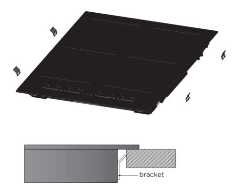
Under any circumstances, the brackets cannot touch with the inner surfaces of the worktop after installation (see picture).
