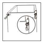
4. Unscrew and remove the bottom hinge pin, turn the bracket over and replace it.
