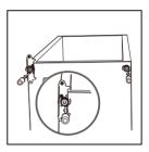
6. Unscrew right middle stopper with metal block from bottom of upper door. And then install left middle stopper and metal block in left side of bottom of upper door. (The same operation as for lower door.)
