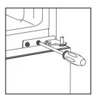
3. Laying down the refrigerator, take out the adjusting feet as below, then unscrew the lower hinge by cross screwdriver.
