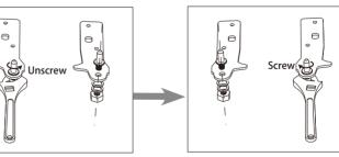
9. Install the hinge at left side and foot base at right side. Then screw two leveling feet with their original parts.
