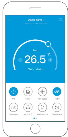
③ Thus, user can control air conditioners on/off status, operation mode, temperature, fan speed and so on.
