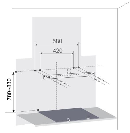
After hang the hood on the installation plate, fasten two screws M5X50, avoid the hood slide off accidently.
