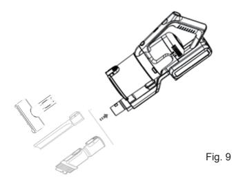
4. To remove the all parts press the release button and accessories firmly pull apart.
