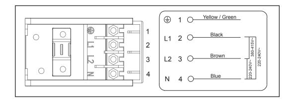
If the total number of heating unit of the appliance you choose is not less than 4, the appliance can be connected directly to the mains by single-phase electric connection, as shown below.
