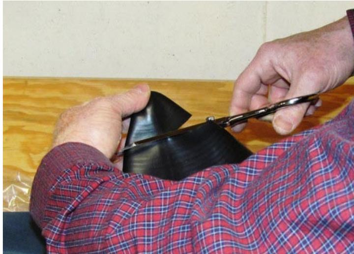
If the gasket has a closed end, cut it off with the scissor above the first molded guide ring (i.e., the smallest opening). This cut doesn't have to be terribly neat, as long as you don't leave any nicks in the edge that could turn into tears when you stretch the gasket in the next step.
