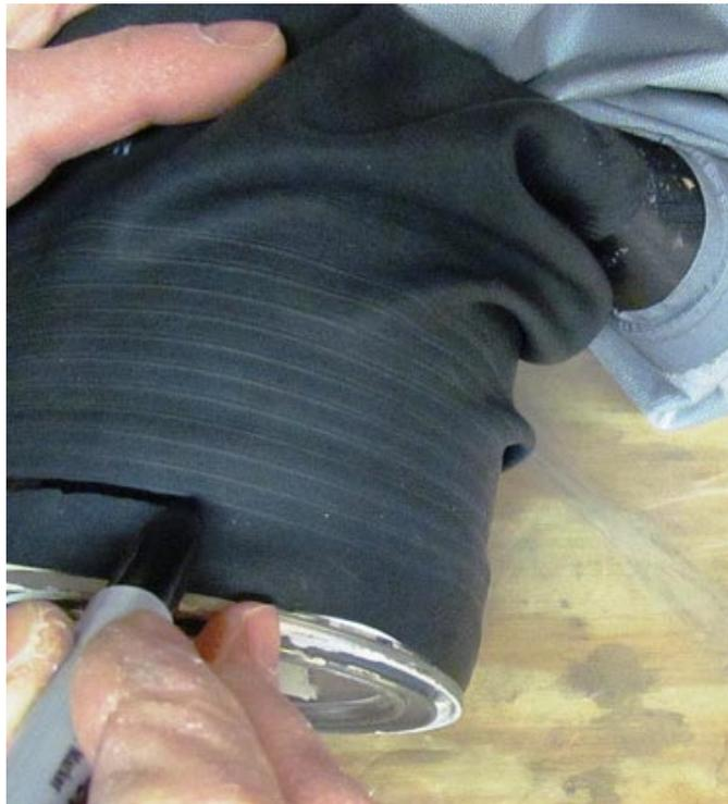
Turn the drysuit inside out. Stretch the gasket over the can and position it so that the guide rings are fairly straight and even. Pick the guide ring you want to cut, and use the marking pen to highlight it all the way around. The guide rings can be difficult to see, even with good light, and the marking pen helps a lot. You can mark just above the ring you plan to cut, or mark right on the ring itself.
