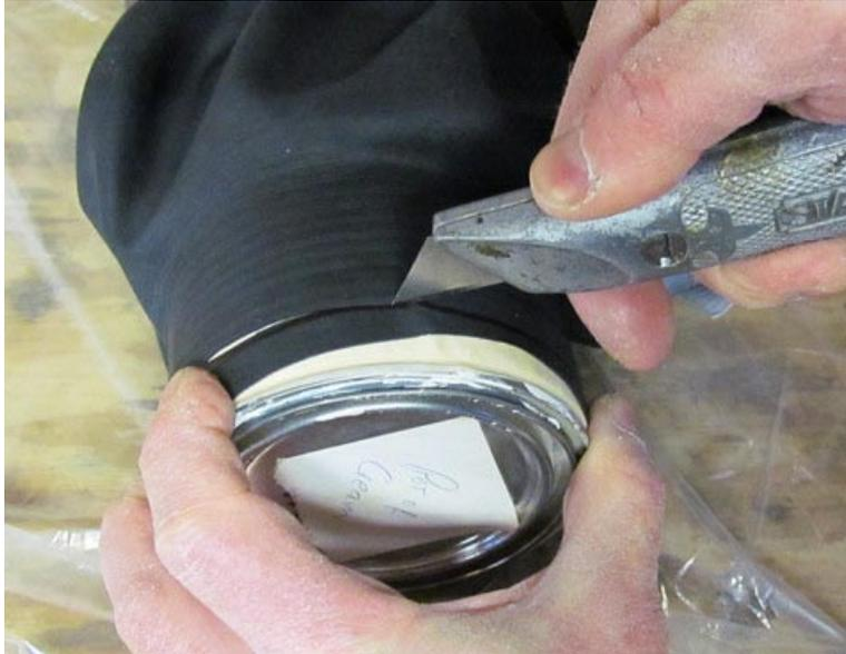
Lay the can on its side. Cut through the gasket with the utility knife, making long, smooth cuts. You'll have to stop periodically to turn the can. When you do, begin the next part of the cut exactly where the previous one ended. Make sure the final cut ends exactly where the first one begins.
