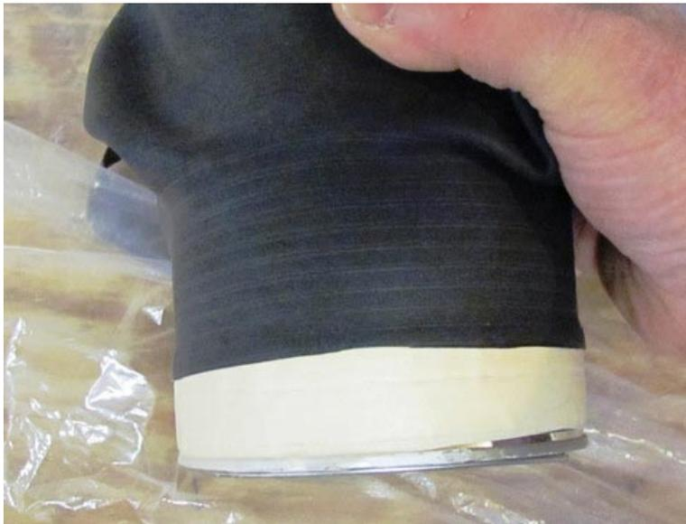
There's a slight dip in the edge of this gasket. This is okay, but if you want to make this a neater job, or if you left a nick in the edge that could turn into a tear, you don't have to cut all the way down to the next guide ring. Instead, make a gradually-sloping cut to exclude the just the flaw. You're aiming for a smooth, gradual dip in the edge.
