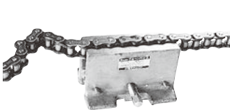
Fig. 3 Setting the roller chain in the chain vise
