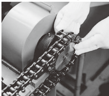
Fig. 8 Connecting on a sprocket
