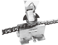
Fig. 2 Grinding the pin ends
