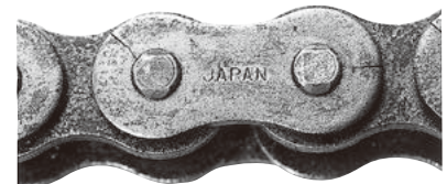
Fig. 32 Hydrogen embrittlement cracking
