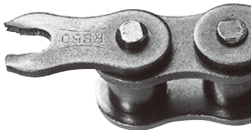
① Static fracture Pulling the link plate with a tensile load beyond its breaking load will cause it to stretch and then break.
