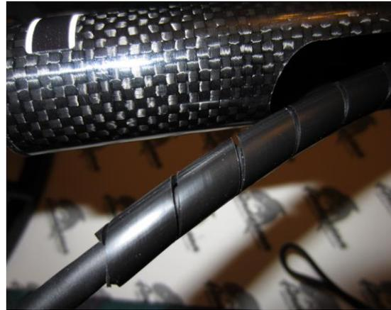
Attach the included pieces of spiral cable protector to the coil cable where it enters the lower rod by simply winding the spiral protector around the coil cable. The spiral wrap should also be applied around the coil cable where it exits the rod for about 6 inches.
