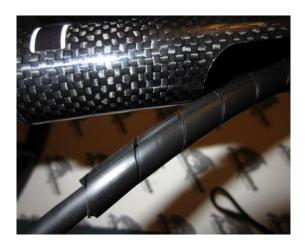
Attach the included pieces of spiral cable protector to the coil cable where it enters the lower rod by simply winding the spiral protector around the coil cable. The spiral wrap should also be applied around the coil cable where it exits the rod for about 6 inches.
