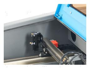
Once set, place a piece of tape on the 2nd mirror's frame. **DO NOT** place the tape directly onto the mirror. Repeat the steps from §5.3.1. If the laser is not centered on the 2nd mirror, you will need to adjust the 1st mirror's set screws accordingly. For larger adjustments, you may need to loosen the mounting bolts at the mirror's base to slide it into better position before fine tuning with the adjustment screws.
