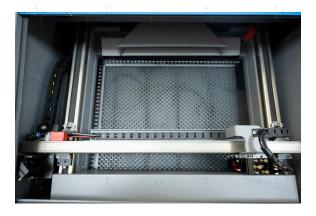
Once set, place another piece of tape on the 2nd mirror's frame. **DO NOT** place the tape directly onto the mirror. Repeat the steps from §5.3.1 and, if necessary, adjust the set screws on the 1st mirror. Test again until the beam is well aligned and retighten the nuts on the set screws.
