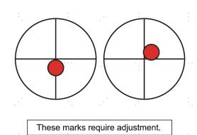
The laser mark should be near the center of the hole. If the laser is not centered on the 1st mirror, cut the power to your laser and carefully adjust the laser tube in its brackets. This may require loosening its fasteners. Be careful not to overloosen any bolts and not to overlighten them. Only adjust one stand at a time.
