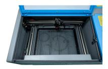
Place a sacrificial base first, preferably a non-reflective steel sheet. Place your laserable material under the laser head and on top of the base, adjusting the base's thickness to make sure the upper surface of the laserable material is at the correct height.
