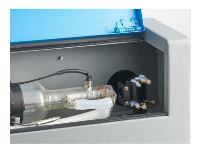
**DO NOT** place the tape directly onto the mirror. Turn on the machine and set the power level to 11% or lower.
