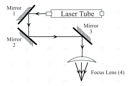
You will need to place a piece of tape at each stage of the laser path, marking it to confirm that that stage remains correctly aligned. When it is not, you will use the laser tube's brackets or the screws on the back of the misaligned mirror to correct the problem. Once the provided tape runs out, we recommend masking tape as it is easy to manage and use.
