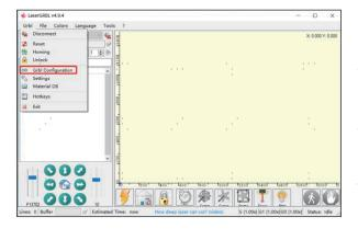
In the configuration menu, change Step Direction Invert (Item #3) from 1 to 3 and Homing Direction Invert (Item #23) from 3 to 1.
