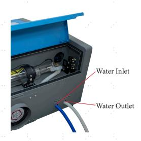
Connect the water pump to its power supply. For best results, use a power outlet on a separate fuse from the engraver itself. If no such outlet is available, the pump can also be plugged into a dedicated socket located on the back of the engraver. Once the plug is plugged in, water should begin to run through your machine and back into your tank. **ALWAYS** obtain visual confirmation that the water is flowing through the laser tube before starting your laser.
