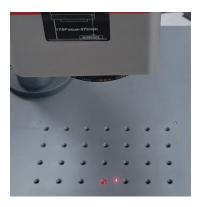
5. Insert the key and turn it clockwise to activate the laser.
