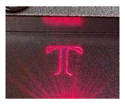
2. Place a piece of laserable test material to display the design at the desired engraving position.
