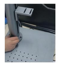
2. Insert and tighten 2 screws to fix the support column by using the provided hex wrench.
