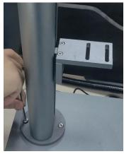
3. Place the laser arm on the mounting bracket of the support column and align the holes on the laser arm with the holes on the bracket while confirming that the scanning head is above the center position of the processing area.
