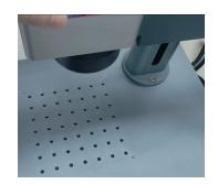
4. Insert and tighten 4 screws to fix the laser arm by using the provided hex wrench.
