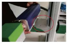
Mount the laser arm so that its lens box is positioned over the work area.
