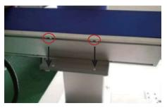
Align the four holes on the housing with the holes in its mounting bracket.
