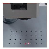
5. Insert the key and turn it clockwise to activate the laser.
