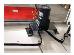
3. The motor is a two-phase 4-wire motor. Use a multimeter to confirm which wires are A+, A–, B+, and B– although these are usually color coded red, green, yellow, and blue respectively.
