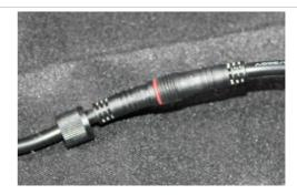
7. Twist the circular lock to keep both connectors in place and waterproof.
