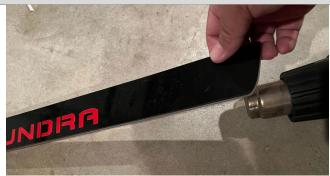
\*\*\*Do no OVER HEAT the sills and do not HEAT up the LED. \*\*\*
