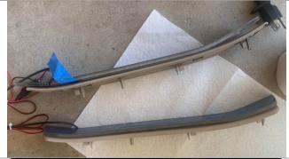
6.  $extstyle{ iny Peel back 1/4 of the double side tape and}$ position the new door sills on the car door.
