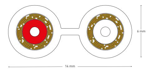
Outside diameter 6 x 14 mm  $4.0 \text{ mm}^2$ Conductor area
