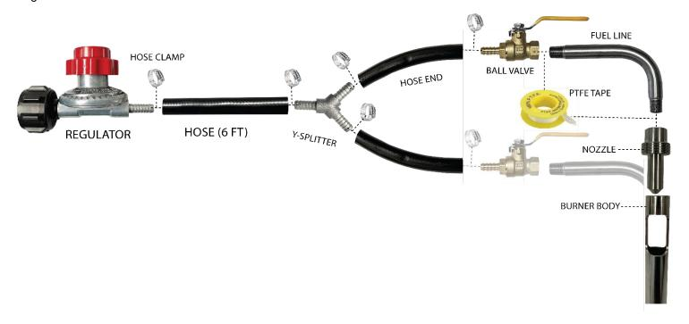
**Hose Assembly**: Connect the propane hose to the regulator, Y-splitter, and ball valves using the hose clamps. Make sure to follow the diagram of the Y-splitter position.
