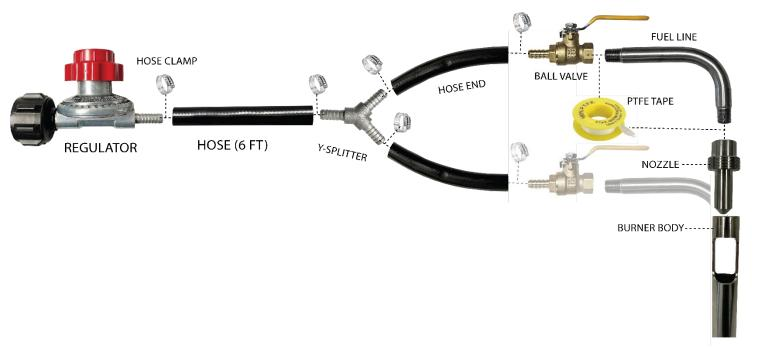
**Hose Assembly**: Connect the propane hose to the regulator, Y-splitter, and ball valves using the hose clamps. Make sure to follow the diagram of the Y-splitter position.
