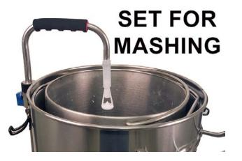
Too much flow, and the unit will run dry (you will hear a sucking sound) and too little, and the needed 1" of liquid above the grain will not be maintained. You will have to play around with the valve adjustment a bit to maintain about an inch of water above the grain bed as every mash is different.
