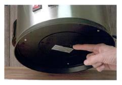
**ER4:** Thermostat overheating protection. This can happen when the heating element and thermostat are covered by a hop or grain bag. It can also be caused by heavy trub deposits resulting from too fine a grain crush, or malt extract or honey being poured into the unit, coating the thermostat. Reset by unplugging, and pressing the reset button on the bottom center of the unit.
