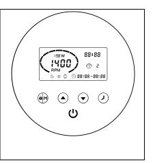
Once the pump has finished priming, the inverter will automatically switch the pump to the pre-set speed, (INDIA) indicates the pump is running and showing current rpm and power consumption.
