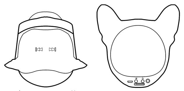
Remarks: Long press  $\bigcirc$  to turn on/ off the speaker, button  $\bigcirc$  switches modes. Short press  $\bigcirc$  or  $\bigcirc$  change songs. Under Bluetooth mode when the 3.5mm audio plug is inserted in, the speaker will switch to line in status.
