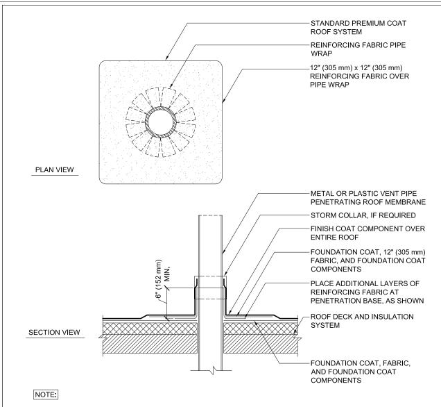
1. THIS DETAIL IS A TYPICAL PENETRATION DETAIL APPLICABLE FOR ALL COLD PIPE PENETRATIONS. FOR HOT PIPE PENETRATIONS, CONTACT THE MANUFACTURER FOR REQUIREMENTS.
