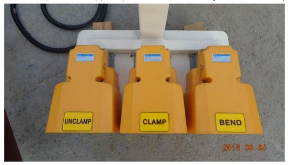
Press the following circled button to bend position, the bending leaf will up and bend, after bending put the circled button to release position, the bending leaf will down and loose.
